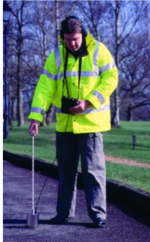
Omikron \gamma ground microphone in use
