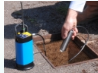
Use of separate accelerometer
