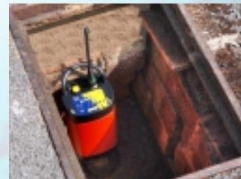
Internal accelerometer connects direct to pipe
