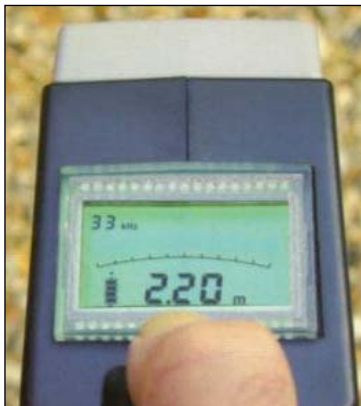
LCD meter displays signal strength, mode, depth and battery
